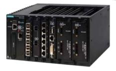
The RUGGEDCOM RX1510 have an IP30 degree of protection, do not use internal fans for cooling, can withstand high levels of electromagnetic interference, and support a wide temperature range of -40 °C to +85 °C. The modular and field replaceable platform allows customers to select amongst WAN, serial, and Ethernet options, making it ideally suited for electric power utilities, the industrial plant floor, rail and traffic control systems.
